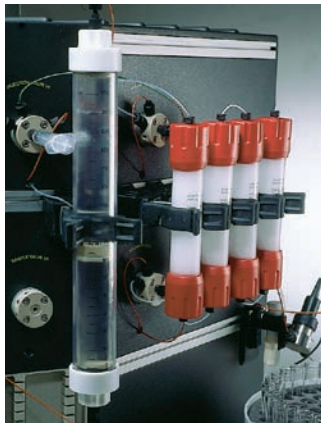
Fig. 51. Four HiPrep 26/10 Desalting columns connected in series.
