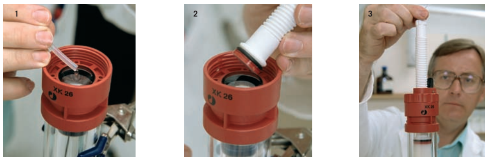
Fig. 70. Adding the top adaptor.
