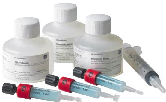
Fig 32. HisTrap FF crude Kit provides convenient and simple purification of histidine-tagged proteins.
