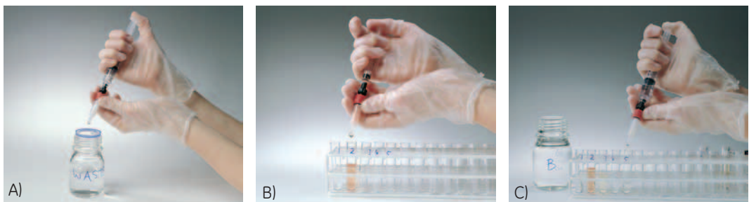
Fig 57. Using a GSTrap column with a syringe. A) Prepare buffers and sample. Remove the column's top cap and snap off the end. B) Load the sample and begin collecting fractions. C) Wash and elute and continue collecting fractions.
