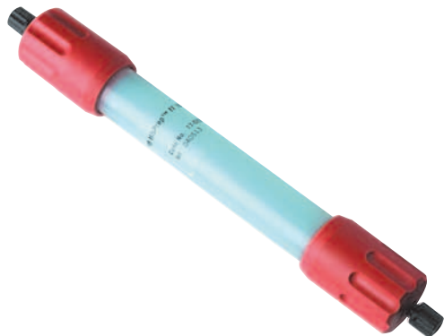
Fig 37. HisPrep FF 16/10 column for convenient scale-up purification of histidine-tagged proteins.
