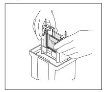
5e. Lower the Inner Chamber into the Mini Tank. Fig. 5. Mini-PROTEAN 3 assembly.
