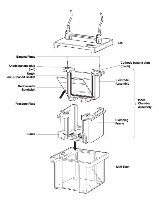
Fig. 2. Assembling the Mini-PROTEAN 3 cell.
