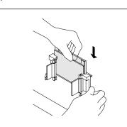
4b. Slide the two plates into the Casting Frame keeping the Short Plate facing front.
