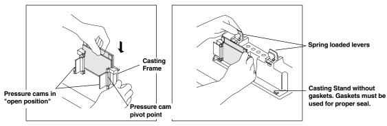
Fig. 3. Assembling the Mini-PROTEAN 3 Casting Frame and Casting Stand.
